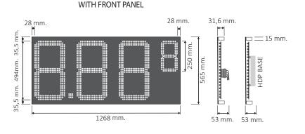
Model Code Details HDP50P-A-WSMD-4 D 100 2557 With Front Panel, White LED HDP50P-A-RSMD-4 D 100 2558 With Front Panel, Red LED HDP50P-A-ASMD-4 With Front Panel, Amber LED D 100 2559 HDP50P-A-GSMD-4 D 100 2560 With Front Panel, Green LED HDP50P-B-WSMD-4 D 100 2561 Without Front Panel, White LED HDP50P-B-RSMD-4 Without Front Panel, Red LED D 100 2562 HDP50P-B-ASMD-4 Without Front Panel, Amber LED D 100 2563 HDP50P-B-GSMD-4 D 100 2564 Without Front Panel, Green LED
